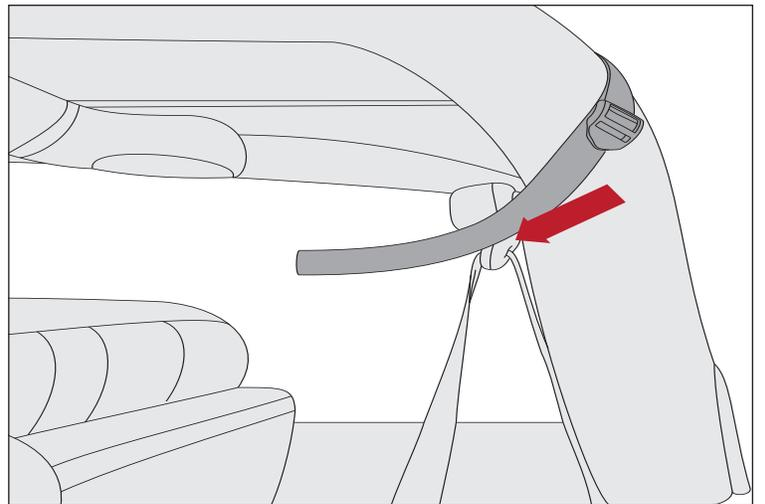
14. Loop strap under seatbelt stud, then back around to outside of vehicle.
