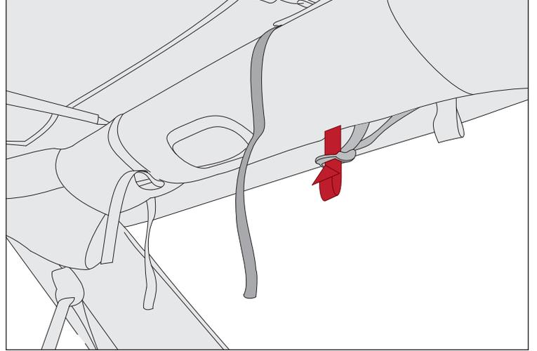
13. Loop rear side strap around rear sport bar, moving toward outside of vehicle.
