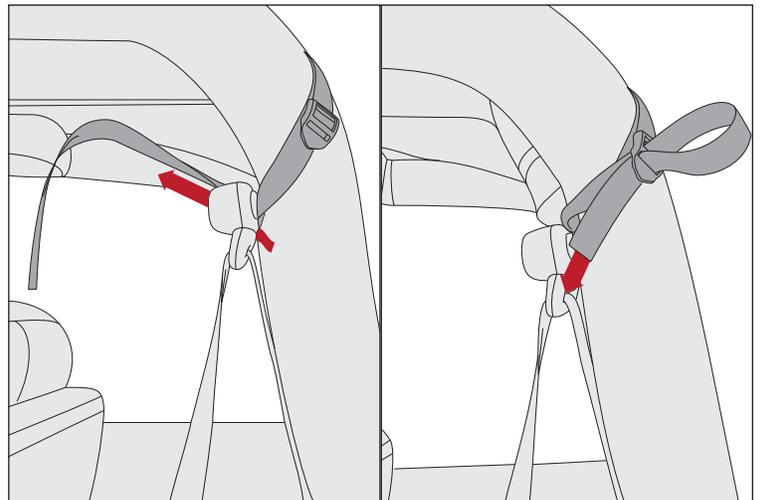
15. Loop strap through plastic buckle and pull strap to tighten. Repeat for opposite side.
