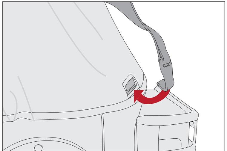
28. If desired, rear window can be rolled upwards, secured with two rear straps, and fastened to top with snaps located under top flap.
