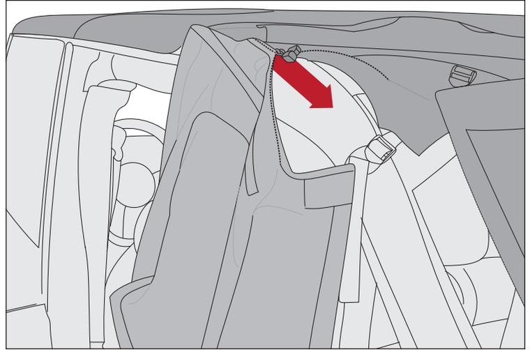
21. Pull bottom plastic retainer of side window into side groove of body tub. Repeat step 19 - 21 for opposite side.
