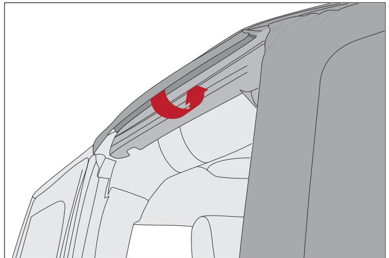
10. Pull two center straps on inside of vehicle around sport bar.
