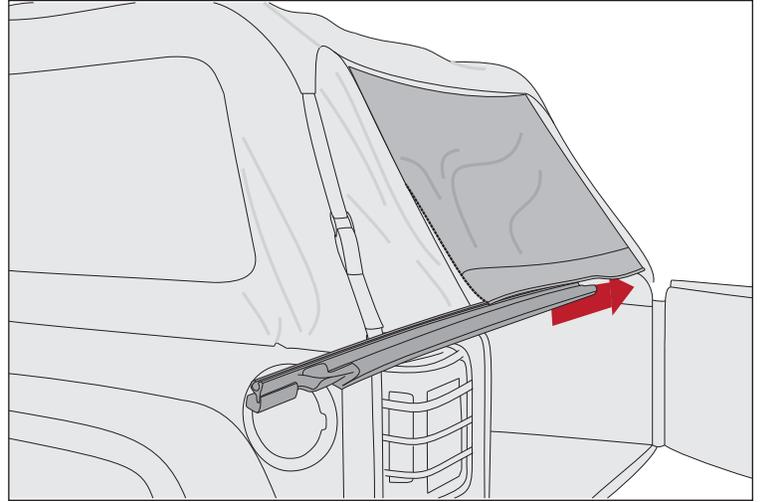
27. Install metal hook on end of rear straps into body tub through cutout in rear panel and tighten. Repeat for opposite side.
