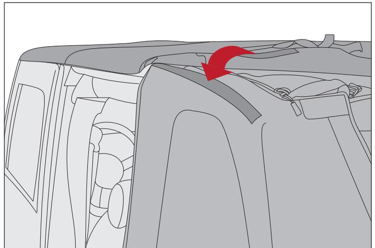
25. Insert remaining side window plastic retainers into groove of body tub. Repeat for opposite side.
