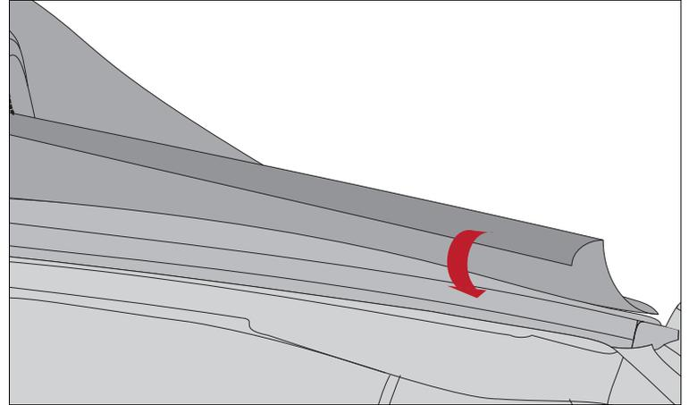
7. Locate ceiling adjustment straps at rear corners on ceiling panel. Gently pull strap over rollbar and around seatbelt stud and back up to strap adjustment buckle. Tighten snugly and repeat other side. Check top for evenness from side to side.
