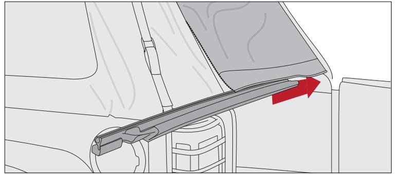
12. On top of rear part of roll bar, pull side to side adjustment straps snug, do not over tighten. Pull three rear window straps snug.
