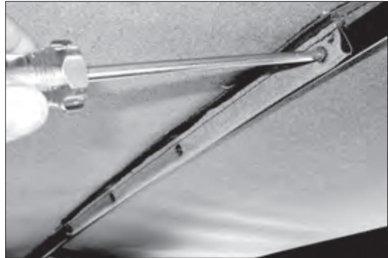
10. Reattach screws that secure top to bow above roll bar. Reattach cable spring to center bow using needle nose pliers and replace fabric spring cover.
