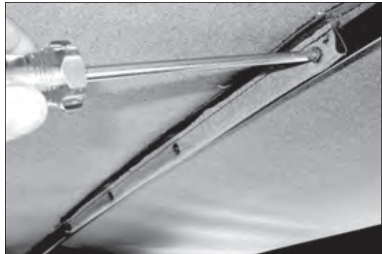
4. Remove screws that secure top to bow above roll bar and set aside for later use.
