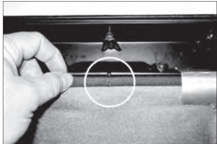
8. Drape new fabric over back of vehicle and lower frame assembly. Wrap fabric around corners of header assembly. Ensure fabric is tucked between lip of header as shown. Reattach plastic tab to header using screws removed in step 5.
