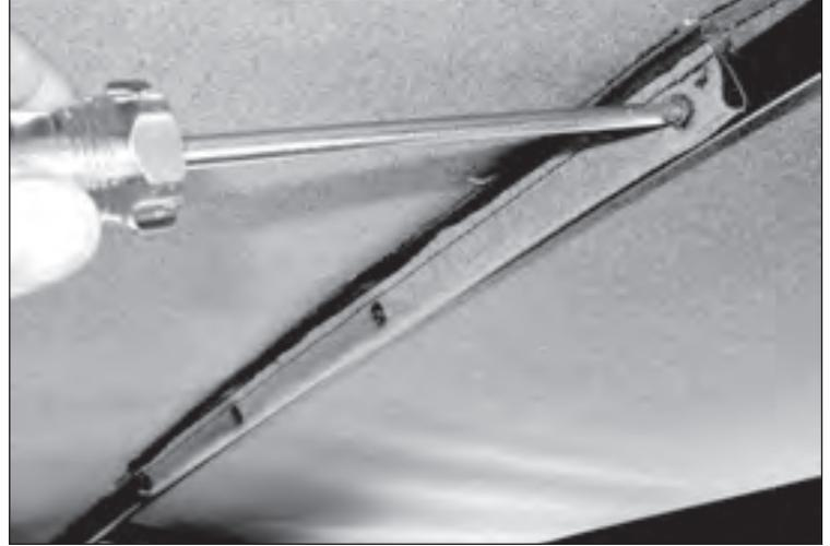
10. Reattach hook and loop retainer around front bow above center roll bar.
