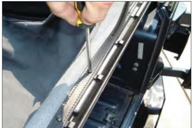
8. Wrap fabric over header and drape it over tailgate. Raise header slightly and work pockets in fabric over corners of header. Install screws removed in step 5 in corners of header.
