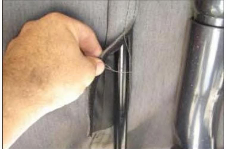
4. Release soft top snaps from rear bow and allow bow to drop on tailgate.
