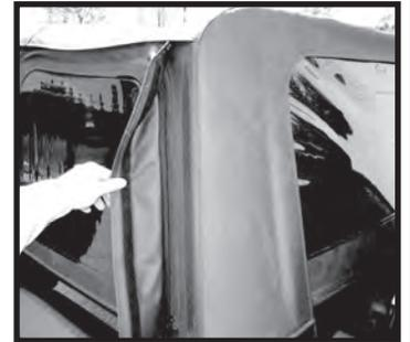
Step 2. Release the rear corners of the top. Pull down and out on the rear corners to remove the fabric from the belt rail. Repeat this procedure for both sides.
