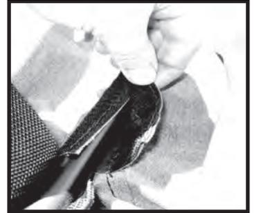
Step 11. Insert the rear corners of the soft top into the belt rail on the rear of the vehicle.
