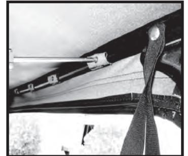
Step 4. Unfasten the hook and loop retainer that secures the top to the bow located above the roll bar. It may be necessary to lower the top at this time to aid in the removal.
