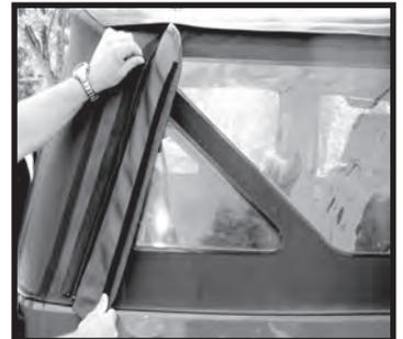
Step 13. Secure the top above the doors by inserting the plastic retainer strips into the door surround. Your new top installation is now complete.
