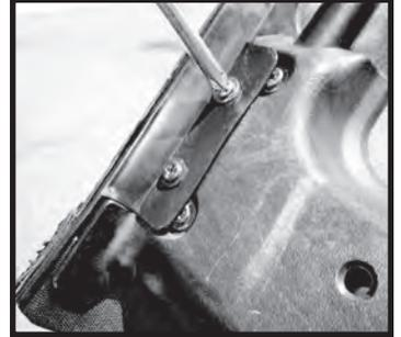
Step 6. With the assistance of a second person, raise the top and bow assembly in the up position. Lock the header to the windshield. Carefully drape the top over the windshield onto the hood. With the top portion of the header exposed remove all of the screws from the top side of the header. Remove the top portion of the header. Remove the old top from the header.
