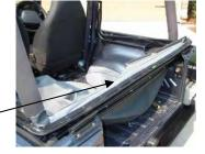
Lay the top fabric, backing side up in the rear of the vehicle with the plastic strip facing up and aligned with the front edge of the header. Locate the round hole that marks the center of the plastic strip (all other holes are slotted). Install a screw in the round hole to secure the fabric to the header as well as to center the top. Then proceed to install screws in the remaining seven or thirteen holes along the front of the header.
