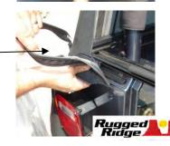
**Step (14):** To start the zipper, pull the two sliders as far down as possible on the driver's side of the window in order to catch the sliders to the pin.
