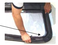
**Step (18):** Reinstall the upper doors. Insert the pins into the grommets in the lower door.
