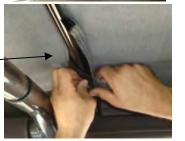
**Step (8):** Locate the left and right quarter window panels and orient them with the zipper slider about 10" - 12" along the top.
