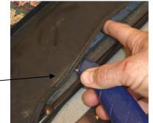
Step (16): Unzip the windows and separate the hook and loop fasteners on the door covers Lay the door cover on a flat surface with the outside facing down. Start by working the lower rear corner of the door frame into the pocket in the lower rear corner of the cover. Then work the lower front corner of the frame into the cover. Work the top front corner of the frame into the corner of the cover, between the hook and loop flaps (not between the zipper and the flap).
