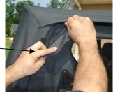
Step (12): Remove the rear window from the box and lay it flat with the backing side up. Locate the tailgate bar set aside in step one. The bar has a "C" shaped channel, when viewed from the end. Orient the bar with the round seal down and slide the "C" channel on the retainer onto the tubed strip sewn to the backing side of the rear window.
