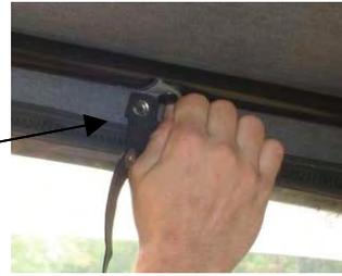
**Step (2) :** Insert front top plastic strip into the windshield channel retainer
