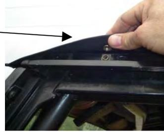
**Step (12):** Unfasten the plastic retainer at the bottom of the fabric door and remove it from the vehicle. Use a razor knife to cut the stitches on the old door covers and remove them from the door frames.
