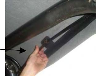
**Step (10):** Open the tailgate. Slide the rear curtain retainer onto the bottom of the rear curtain. Close the rear curtain zippers. Push the rear curtain retainer into the top of the tailgate retainer. Slip the plastic on the bottom of the corners under the bottom fo the tailgate retainer.
