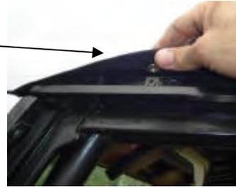
**Step (12):** Unfasten the plastic retainer at the bottom of the fabric door and remove it from the vehicle. Use a razor knife to cut the stitches on the old door covers and remove them from the door frames.
