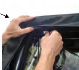
**Step (11):** Fasten snaps on top, above doors, to stubs on vehicle. Studs will slide to match location of snaps on top.
