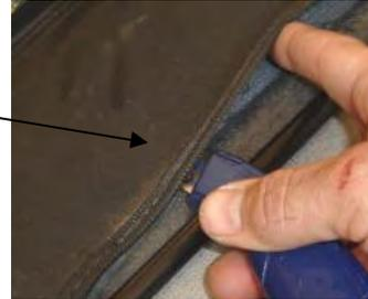
**Step (13):** Separate the hook and loop fasteners on the door covers and slide the new cover onto the frame, starting at the top. Work from corner, to corner wrapping the fabric around the frame and fastening the hook to the loop as you work around the door.
