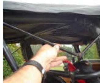
**Step (4) :** Release the rear corners of the top. Pull gently down and then out to release the plastic strip from the retainer on the vehicle.
