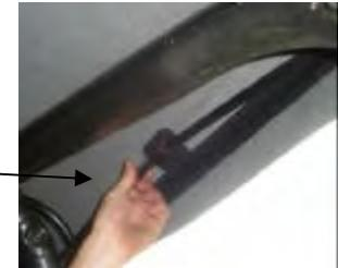
**Step (10):** Open the tailgate. Slide the rear curtain retainer onto the bottom of the rear curtain. Close the rear curtain zippers. Push the rear curtain retainer into the top of the tailgate retainer. Slip the plastic on the bottom of the corners under the bottom of the tailgate retainer.
