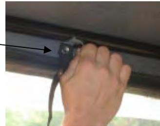
**Step (3) :** Pull down on spreader bars and push rear support bow forward.
