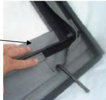
**Step (14):** Reinstall the upper doors. Insert the pins into the grommets in the lower doors.
