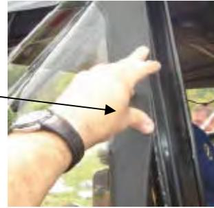
**Step (8) :** Slide the plastic strip on the bottom of the side curtain into the side retainer. Start at one end of the strip and work along to the other end. Close the top and rear zippers on the side curtains
