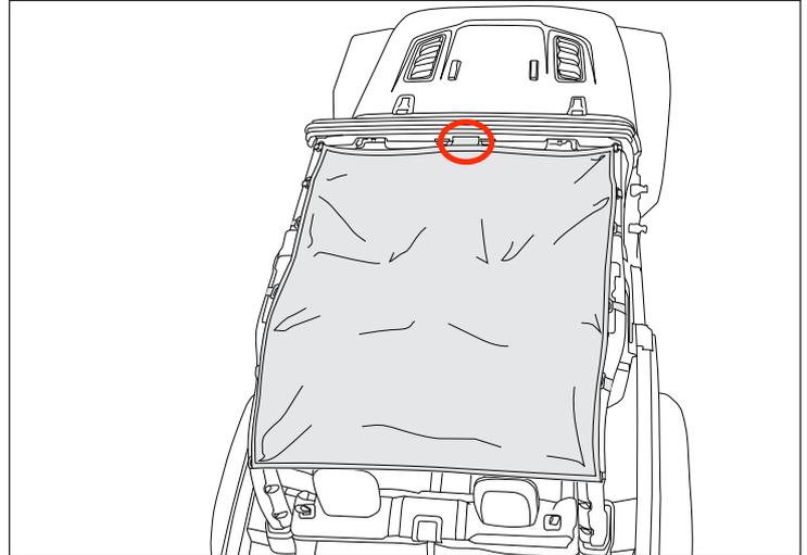
3. Clean center of windshield frame thoroughly with alcohol. Peel and stick Loop Strip to windshield frame avoiding contact with interior plastic panel.
