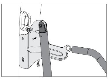
2. Insert Quick Release Bow Knuckles in open ends of soft top bows.
