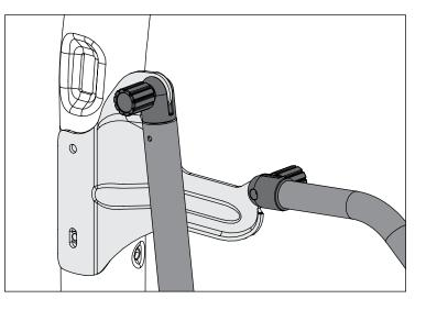
5. Once all bow knuckles are attached to mounting brackets, secure Quick Release Bow Knuckles to soft top bows with factory self tapping screws.
