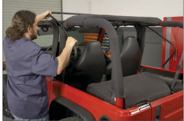
23. Attach the rear bow to the lower pivot point on the roll bar. Attach with shoulder bolt.
