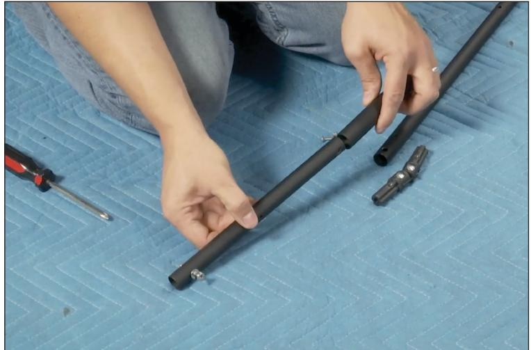
12. Now insert the hinge into the tube and fasten items with a screw. Slide the other end of the hinge into the larger "Dog Leg" tube frame piece. Align the predrilled holes and fasten with screw.
