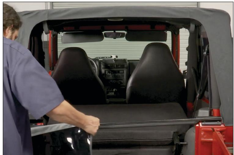
39. Give the sail panels a final tug towards the rear window area. Next zipper rear window into the soft top. Make sure your not just pulling the zipper around but assisting it by pulling the surround material towards the zipper to relieve some tension.
