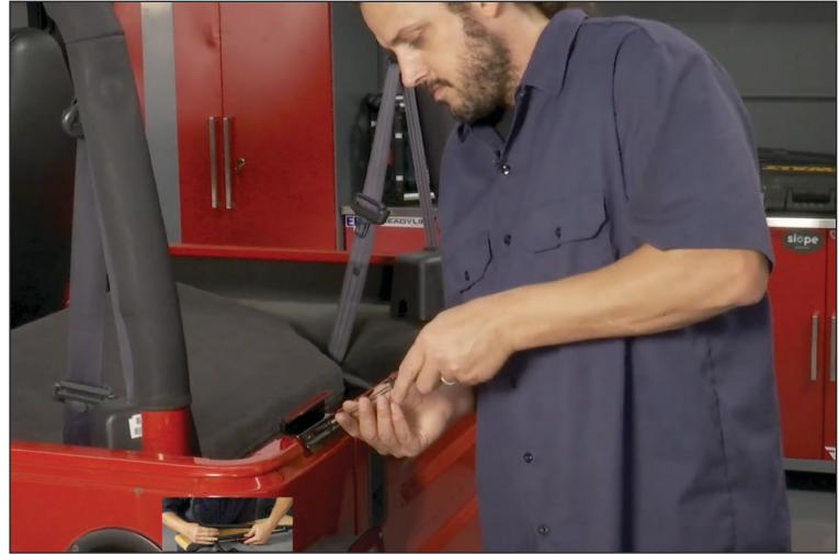
20. Now attach the roll bar bracket to the Jeep. You'll first need to unzip the roll bar pad to expose the attaching location. There are two threaded inserts on the roll bar.
