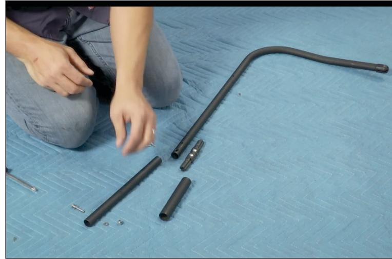
11. Now slide the smaller in length tube over the other predrilled tube. This tube "Locking Bar" is used to slide over the hinge when the top is fully covering the cab to lock out the hinge. To allow for the "Open Air" option of this top you'll slide this tube "Locking Bar" exposing the hinge allowing it to fold the top back.
