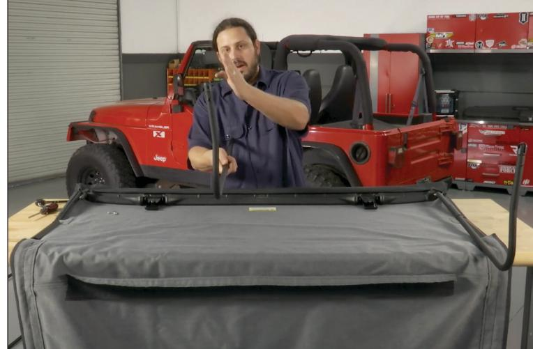
14. Align the predrilled holes and insert the bolt with washer. It's a tight fit and will need to be threaded in. Once bolt is threaded in now place another washer and nylock nut and tighten.
