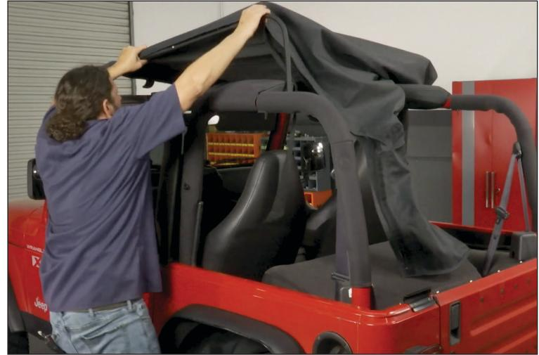
26. Attach the side bow to the upper pivot point on the roll bar and attach with shoulder bolt.
