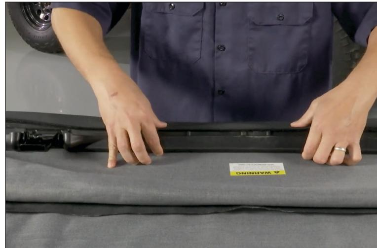
3. Now starting from the center and working your way out screw the top to the header panel. Do not fully tighten until you have all the screws into the header. Pull and adjust as needed to assure the top is center to the header then fully tighten all the screws.
