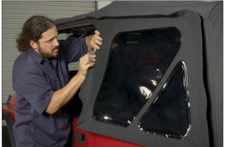
36. Insert lower plastic guide into the Jeep tub rail. Then meet Velcro surface of the window to the top.
