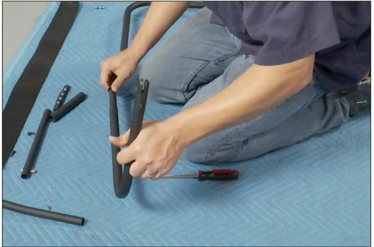
9. Now with the larger "Dog Leg" pieces, they also have plastic knuckles that attach in the same method as the smaller pieces. There is a left and a right side to these items. Notice in the photo how the second slight bend to the tube frame points the tube inwards. This how you determine left to right side. When installing the knuckle the brass insert will be towards the inside. Align the pilot and predrilled holes and attach knuckle with screw.
