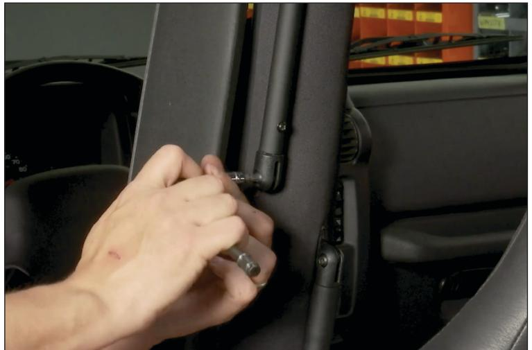
27. Grab the rear bow that sitting in the Jeep tub. Bring it up into position and then grab the center bow straps. This strap attaches to the rear bow with three screws through the strap into the rear bow tube.
