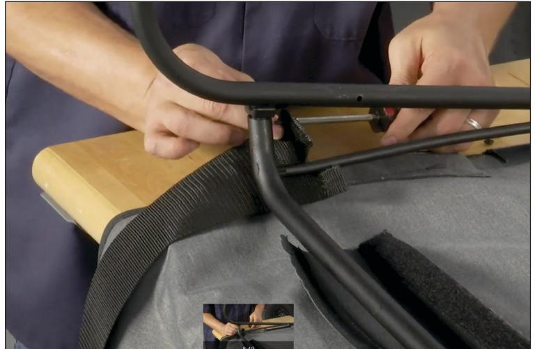
18. With both bows attached to the header and the center bow attached to the side bows, fold a portion of the Velcro and attach to the center bow. Do not attach the entire Velcro just a small portion in the middle to assist in installation. This will allow you the freedom to pull and adjust the top as needed. Once installed and adjusted you'll seal the entire Velcro strip.
