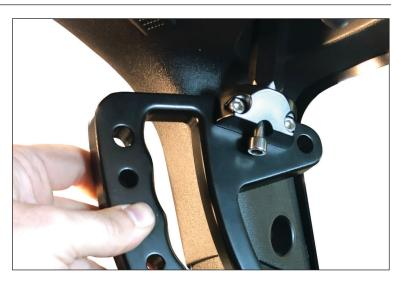
6. Now tighten bolts in a alternating pattern to avoid components from binding up. DO NOT use power tools. Tighten the two bolts snug but do not over tighten to avoid striping the threads or breaking the bolt.
