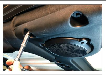
2. Now get the handle and hardware. The kit provides new longer Allen head bolts and hex spacers. Before installing simply thread Allen head bolts in the roll bar to assure threads are clean and free of paint, dirt or burs. Unthread the bolts and now install with the handle.
