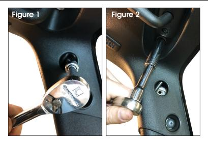
5. The handle requires some preassembly. Use the small allen head bolts to attach the mounting cup to the handle. The cup protion will be to the top of the handle.
