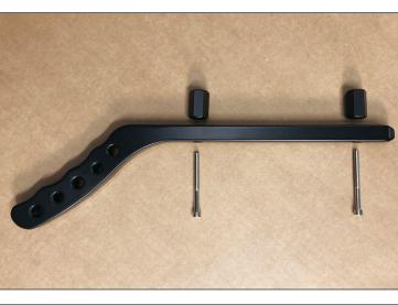
3. Insert Allen head bolt through the handle and then through the hex spacer into roll bar. DO NOT Overtighten the bolts or use power tools to tighten, it could cause the threads to be striped or bolt to break. When tightening alternate between to the two Allen head bolts to assure the handle seats flat to the roll bar.
