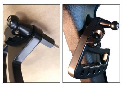
8. Now take the shorter bolt insert into the handle and then the hex spacer while rotating the handle into position. This can be a little tricky to align so take your time to avoid cross treading.
