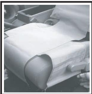
10. Test all seat functions. Hooks and straps should not effect seat movement.
