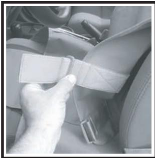
6. If seat is equipped with side air bags make sure straps are clear of deployment zone.
