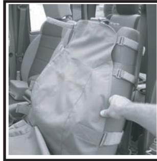
4. Slide front hold down strap between upper and lower seat sections. Reclining the seat will ease strap installation.
