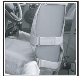
9. Pull sides around seat base and attach retainer hooks to suitable points under seat base.
