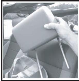
3. Slip cover over top of seat. Pull down into position. Straps should be placed above and below reclining lever if equipped.
