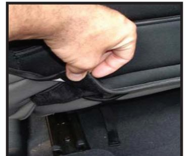
Step 7. Side ABS air bag cover should slipped under cover as shown. Install head rest cover and attach velcro to secure.
