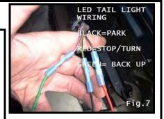
Wiring for the LED Tail Light is as follows:
