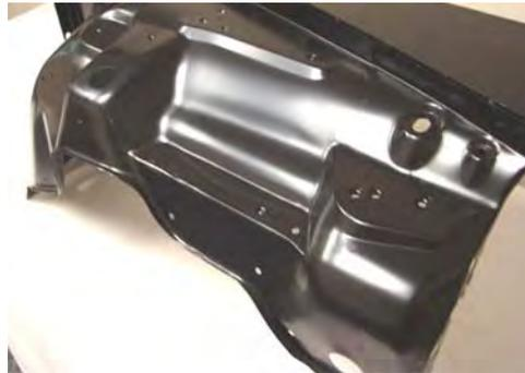
**Battery tray and lower fender support brackets are also retuned to original locations with no drilling and minimal realignment.**
