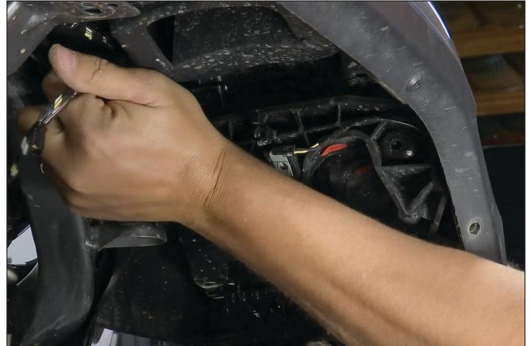
8. Now release all the white retaining clips that attach the fender to the Jeep. Use a small set of needlenose pliers to pinch the back side of the clip and pull the fender from the Jeep. The last clip at the bottom of the fender is deep in the fender. Standard needlenose pliers won't reach it. You could use a long screwdriver or just pull to release this clip. Now fender can be removed.
