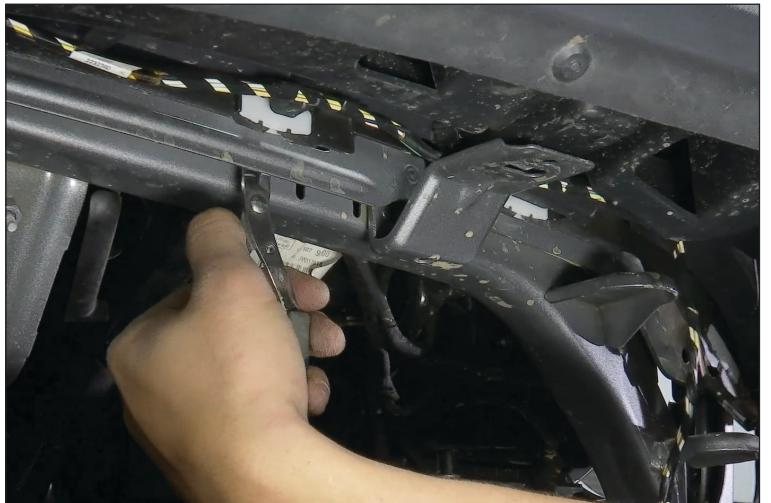
9. Place the fender on a soft surface to assure the paint won't be scratch during modification. First pry and remove all the fender clips to reuse later. Also remove wiring harness from fender.
