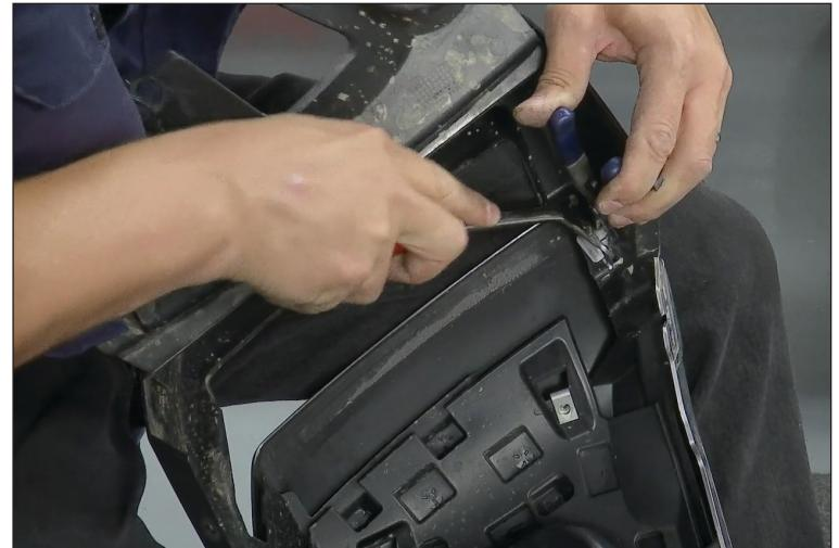
11. Remember to place fender on a soft surface. Now pull the inner fender away from the out fender. These items are glued or fused to each other. Start at the bottom corner of the fender and pry the pieces apart from each other.
