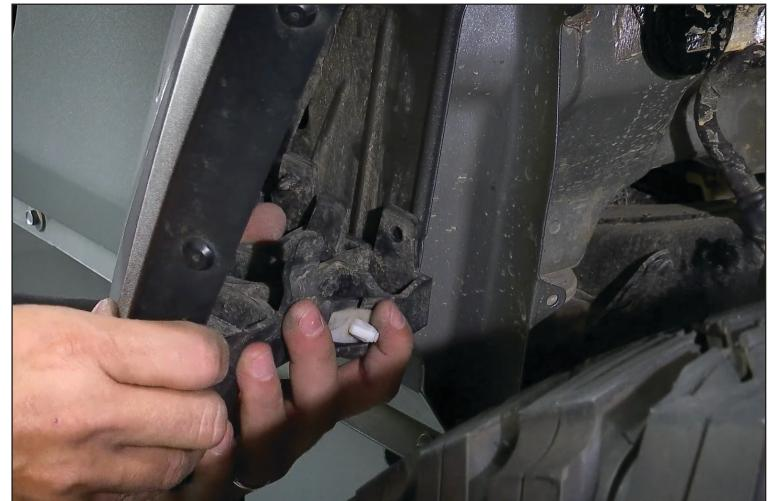
3. Unplug the fender wiring from the chassis harness
