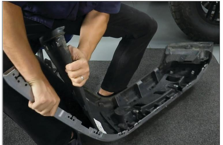
12. The locating tabs need to be trimmed away. A shape box blade works well cutting through the plastic. Feel free to use other tools if you feel fit. Take your time don't rush or force your cut. That could accidentally cause you to cut to far or scratch the paint.
