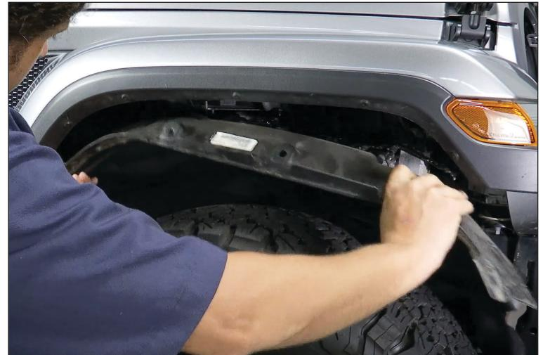
2. Remove the lower fender brace located at the rear bottom of the fender.
