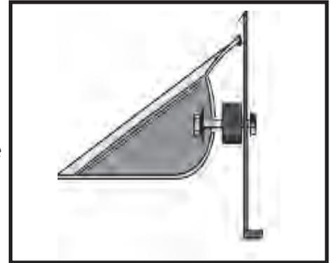
Step 7. Installing the front flares. First you will install the side marker in the flare using two phillips head screws. Install a 7mm rubber spacer on both marker light screws. Install one 7mm rubber spacer on the front mounting screw. Install a 13mm spacer on the remaining mounting screws. Mount the flare on the body placing a M5 nut on each bolt. Finally tighten the side marker screws. Do not over tighten the marker light screws or mounting nuts.
