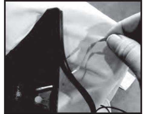
Step 2. Clean inside mounting lip edge with rubbing alcohol. Install edge trim as shown in the figure, removing red vinyl tape covering only a few inches at a time. Do not pull trim while being applied, this may cause shrinkage after installation.
