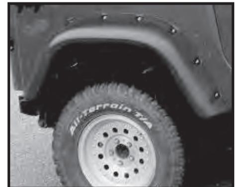
Step 9. Install the front flare extensions using the factory M5 bolts.
