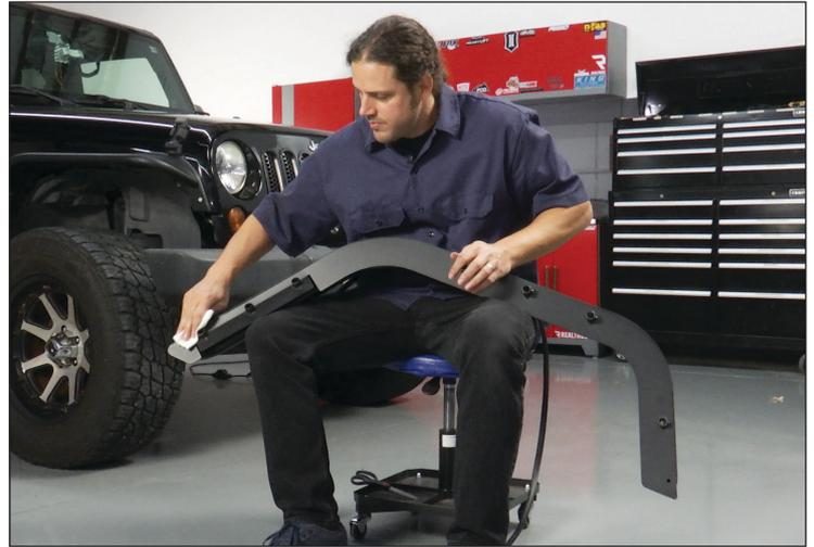
2. When applying the fender seal, peel back a small portion and apply to the fender. Peel and press along the entire top edge of the fender. Once you reach the bottom rear edge of the fender trim seal with a scissors or utility blade.
