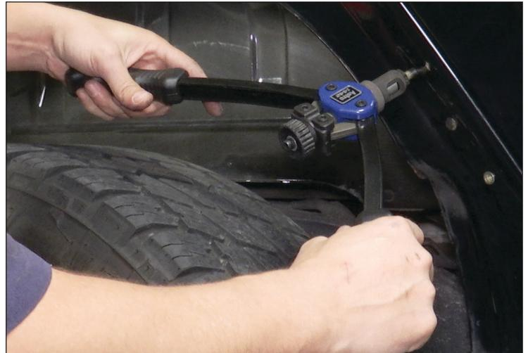
6. To install the nutsert, load tool properly with a nutsert. We recommend applying a small amount of RTV silicone to the edge of the hole to fully seal the nutsert to the body and to avoid water or debris to enter. Insert nutsert into the body of the Jeep and crimp. Take your time crimping to assure it's fully crimped. This will avoid the nutsert from spinning or being crooked.
