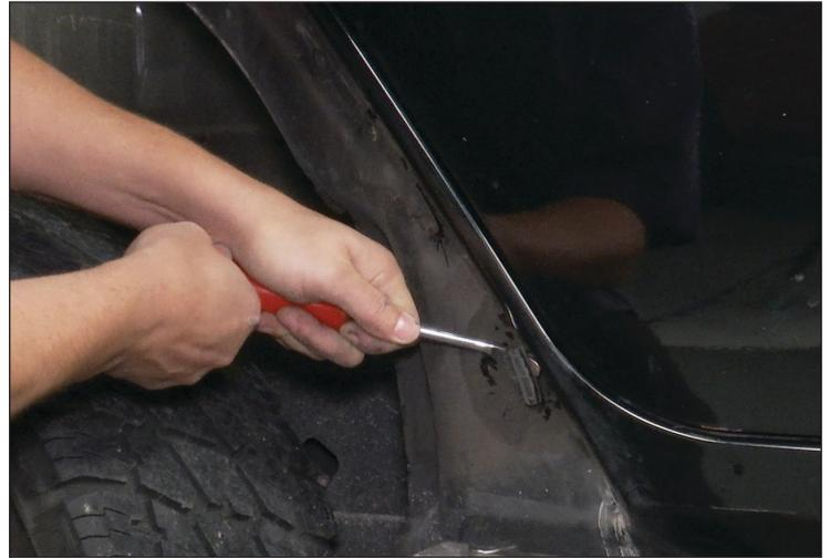
5. The fender is attached to the body using nutserts. There are available at most automotive tool stores or online. We recommend using the tool shown here.
