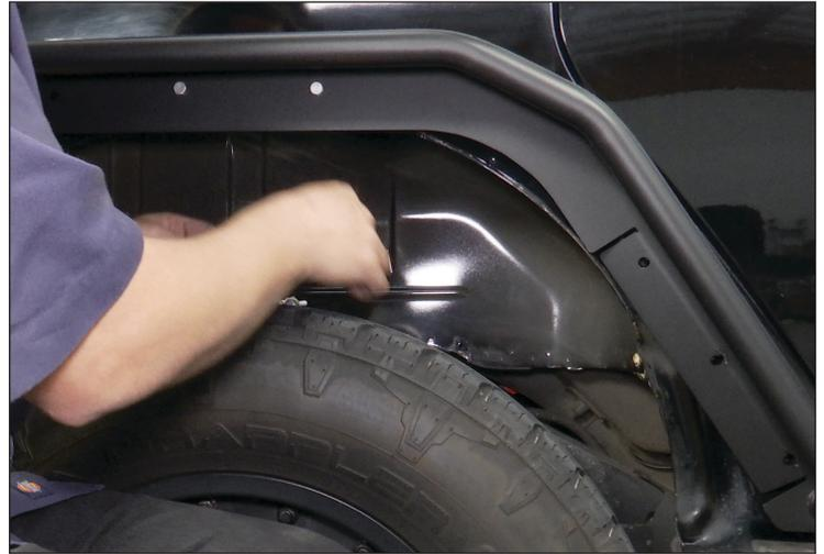
8. Now tread the bolts into the remaining nutserts. Avoid using power or air tools, now tighten all hardware with hand tools in a alternating pattern. That completes the install of your steel tube fenders.
