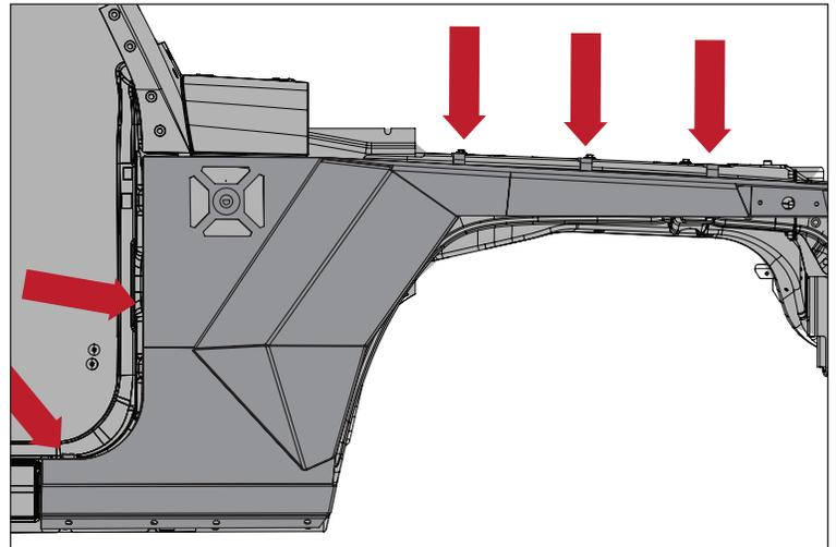
22. Align Upper Cowl and Armor Fenders and tighten Upper Cowl and Cowl Bracket hardware. Use OE hardware to loosely attach Upper Cowl to vehicle.
