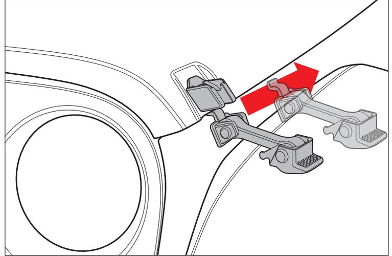
9. Remove Side Marker Bulb and disconnect wire harness, retaining clip from flare.
