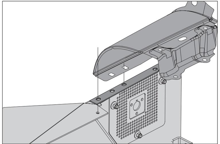
18. Unscrew antenna mast, remove plastic cover, and unbolt antenna base from OE fender.
