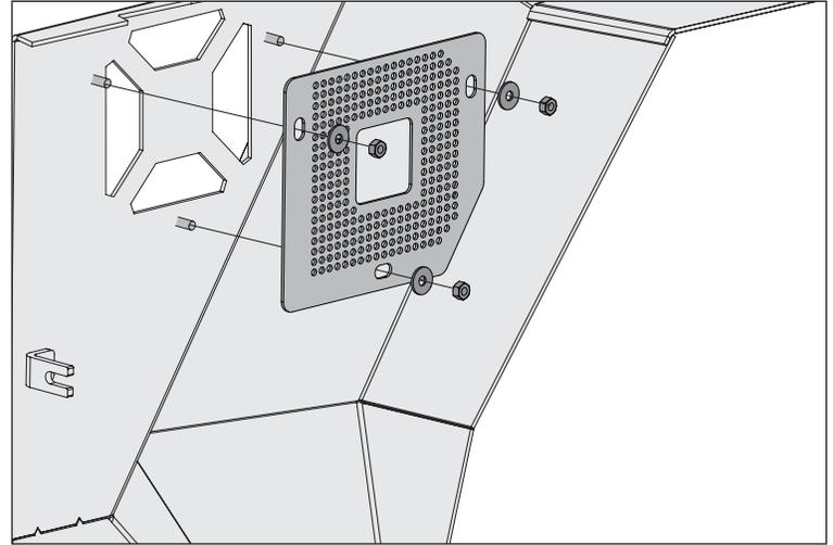
17. Using supplied M6 Stainless Steel Bolt, Washer, and Nut, loosely affix Upper Cowl to Cowl Bracket. Loosely attach Upper Cowl and bracket to Fender Armor.
