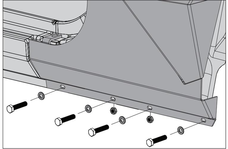
25. Using supplied M8 Hex Bolts, Washers, and Nuts, attach Front Mounting Brackets to Armor Fenders. Using OE bolts, attach Front Mounting Brackets to vehicle.
