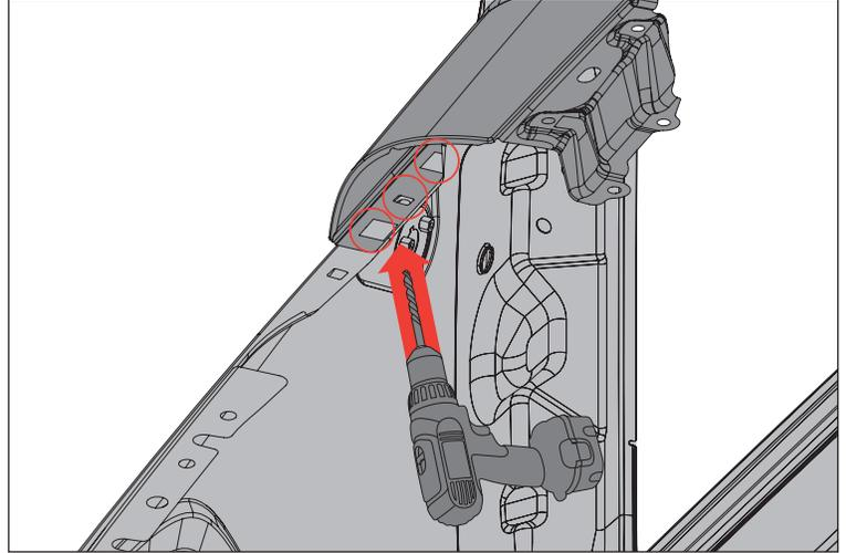
14. Attach supplied Side Marker Lenses, using supplied M4 Socket Head Bolts, Washers, and Nuts to Fender Armor.
