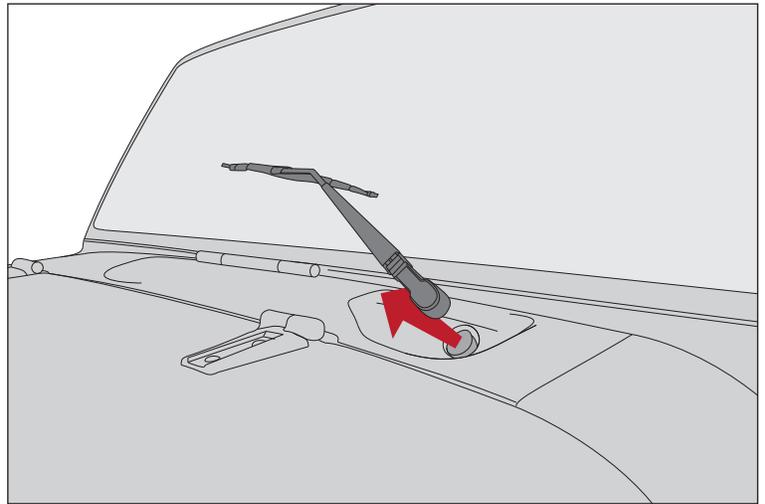
3. Remove cowl screws using T30 socket. Lift hood. Carefully remove cowl center plastic retainer clips using flat head screw driver and carefully remove cowl cover from vehicle. Close hood.
