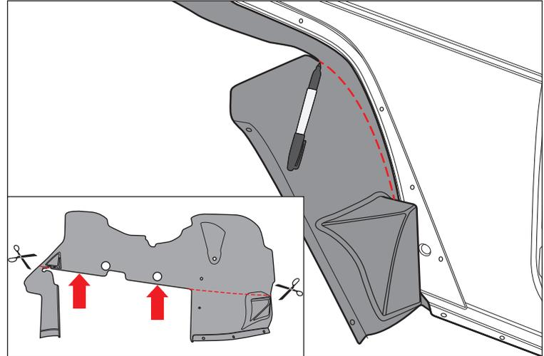
31. Position supplied Rubber Plate next to cut OE fender liner as shown. Cut opening for flare support bracket. Using supplied sheet metal screws, attach Rubber Plate to cut OE fenders. Fold rubber plate into Armor Fender.
