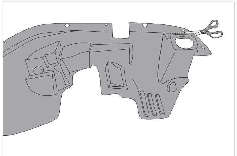
29. Attach Rugged Ridge front fender liner reusing factory bolts.
