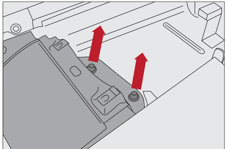
7. Remove 7 inner fender bolts and retain for later use. Remove lower pinch seam bolts.
