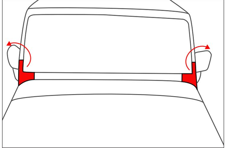
2. Using 13mm wrench, remove both wiper arms.
