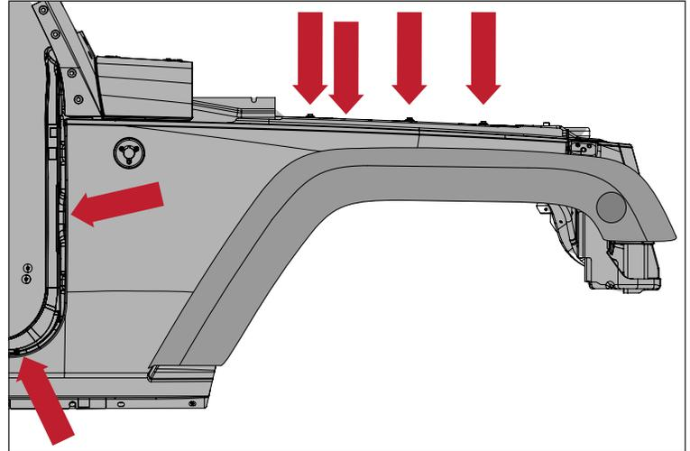
5. Remove two inner cowl bolts located under Cowl Cover. OE bolts will be reused.
