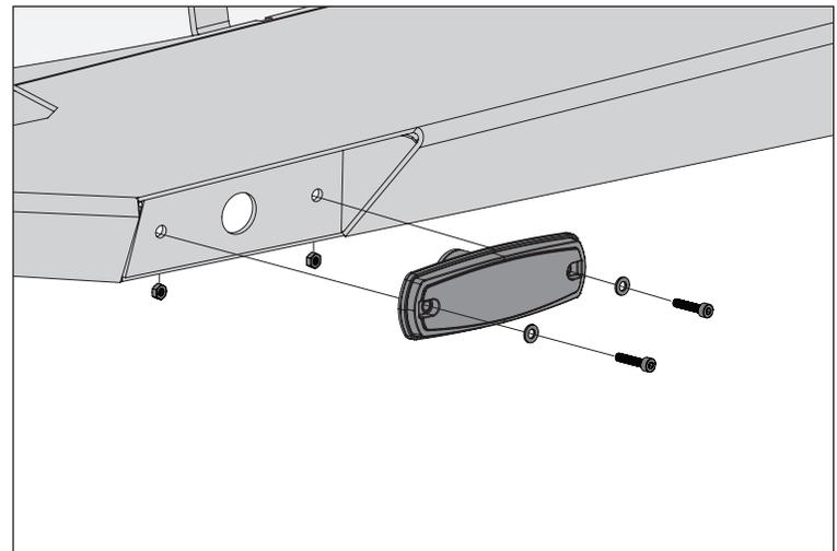
15. Attach Lower Hood Catch to Fender Armor reusing OE hardware.
