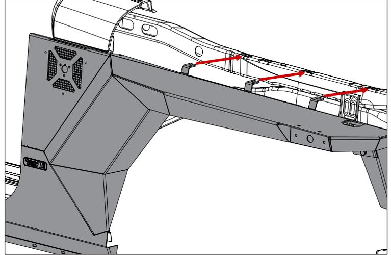
21. Loosely attach Upper and Door Jamb Mounting Tabs to vehicle using OE bolts. Loosely attach Armor Fenders to Flare Mounting Bracket using supplied M8 bolt, washers, and nut.
