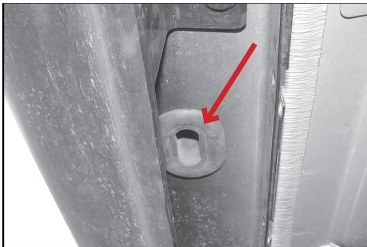
3. Partially thread 12mm Plastic Retainer onto 12mm Bolt Plate.
