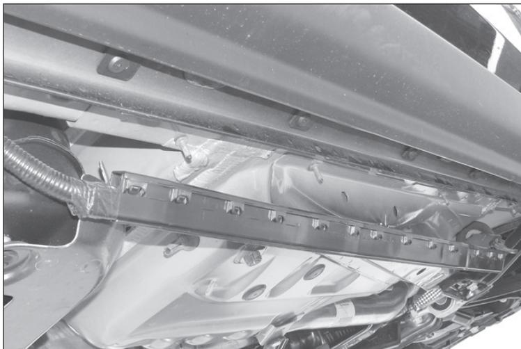
2. Starting on driver side, locate factory holes in pinch weld. Near front pair, remove rubber plug filling oval hole in bottom of rocker panel in front of two holes.
