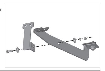
5. Select Passenger/Right Front Support Bracket. Attach Support Bracket to back of Front Mounting Bracket using M8 Hex Bolt, 2 M8 Flat Washers, M8 Lock Washer, and M8 Hex Nut. Line up mounting flange on Support Bracket with back of pinch weld.
