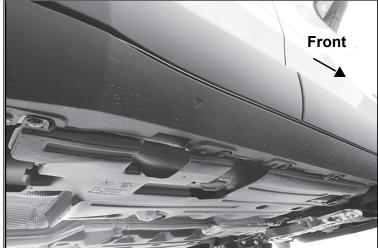
3. Select M10 Bolt Plate. Insert Bolt Plate into hole in frame channel.
