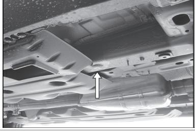
2. Remove long plastic cover from bottom of floor panel. Play close attention to location and type of factory fasteners for installation.
