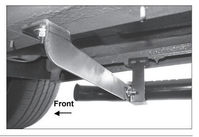
6. Move toward rear of vehicle and locate square plug in bottom of frame channel. Repeat steps 2-5 to install Passenger/Right Rear Bracket and Support Bracket.
