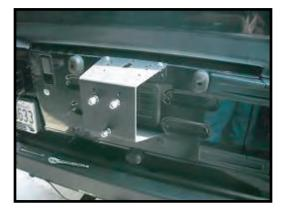
7. If applicable, route third brake light wiring through large slot in top of Tire Carrier, and place brake light assembly on top of Tire Carrier. Use (4) M8 Bolts, (8) M8 Flat Washers, (4) M8 Lock Washers, and (4) M8 Nuts. Once all are in place, tighten them. Re-route wiring and plug it back into contacts.
