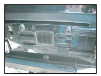
5. Hang the Angle Bracket using original hardware in the top mounting holes. The slots go against the body. Do not tighten hardware yet.
