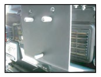
4. Remove original Tire Carrier. Keep the hardware, as it will be reused.
