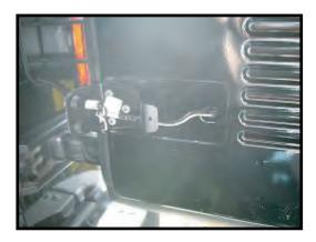
2. Pass Third Brake Light wiring through tail gate. Remove Third Brake Light assembly.
