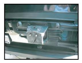
3. Install (3) M12 Bolts and (3) M12 Lock Washers into Tire Carrier Bracket from the back side as shown. For 5 x 4.5" bolt pattern wheels, use the bottom hole, and the two closest to it. For 5 x 5.5" bolt pattern wheels, use the bottom hole and the two furthest from it.
