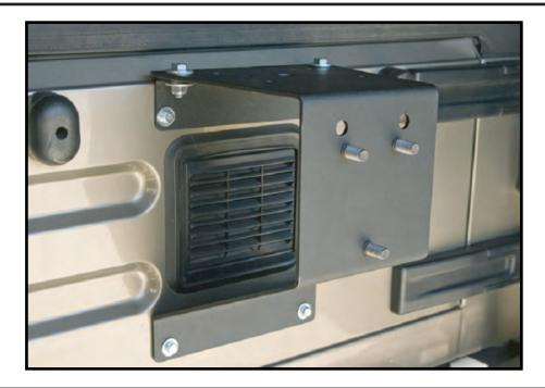
1. Remove spare tire. On vehicles equipped with a third brake light, remove wiring cover inside the tailgate. Note where each wire is attached, then disconnect and route wires out of the cover bracket.
