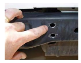
Attach brackets with the (4) 10mm bolts, flat washer, lock washer and nuts supplied for each side. Tighten to 45lbs. **NOTE: ON 97-2006 Wranglers there might be a tight fit between the rear cross member and the fuel tank. A second person to help might be needed.**
