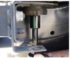
**Step (2)** Locate the left and right bumper mounting brackets. Place left bracket with large vertical tab facing outwards, towards the inside of the vehicle. For 1955 -86 CJ's the holes in the frame crossmember will line up (Use the inner mounting holes on the supplied brackets). temporarily mount the brackets into place.
