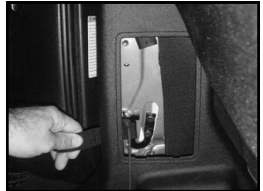
10. Apply Logo to the oval recess located in the lower rear corner of the door. Be sure the surface of the door is cleaned thoroughly and dry before Logo is applied. **NOTICE!** If doors will be painted, do not attach Logo until the last coat is applied and fully cured.
