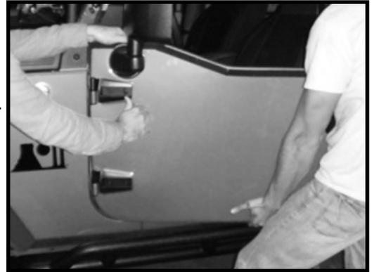
8. Only if necessary adjust the position of the vehicle striker bar for proper latch engagement. Locate the vehicle striker bar in the door jamb on the B-pillar. Loosen bolts and adjust as necessary. Tighten to 19 ft-lbs. **NOTICE!** Any adjustments made to the vehicle striker bar will need to be repositioned upon re-installation of factory doors.
