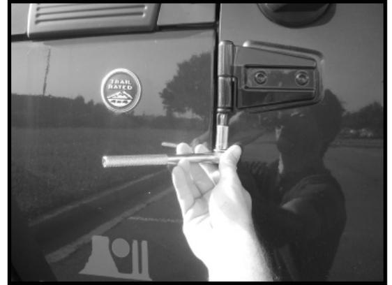
4. Remove (4) temporary bolts from the two hinge locations of each Half Door. Install supplied Door Hinges with the hinge pins pointing downward using the supplied M8 Countersunk Bolts. Tighten to 15 ft-lbs.
