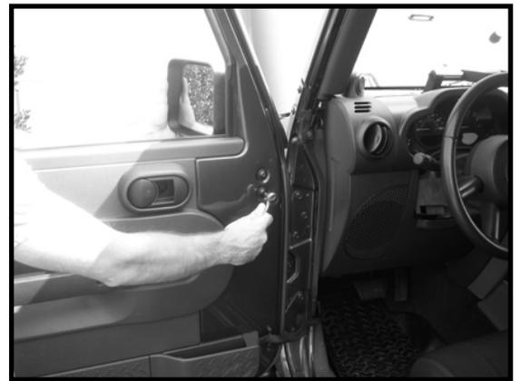
2. Disconnect wiring harness before removing door. Release the red locking tab and pull down on the connector. Next, remove the strap from the hook located inside the vehicle. **NOTICE!** Door can swing freely once the strap is released potentially causing damage to your vehicle. Do not let go of door when strap is disconnected.
