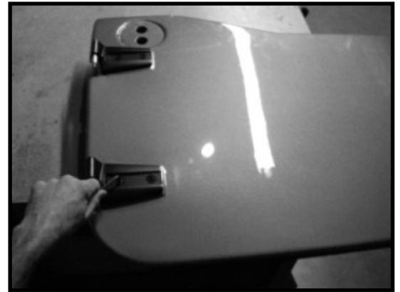
5. Attach the Grab Handle to the door using Grab Handle Mount Plates and M6 Bolts by carefully aligning with threaded hole locations on door.
