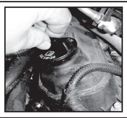
Step 2. Install the new billet oil cap. Reuse factory O-ring.
