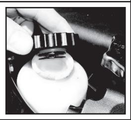
Step 2. Install the new power steering reservoir cap by turning clockwise.
