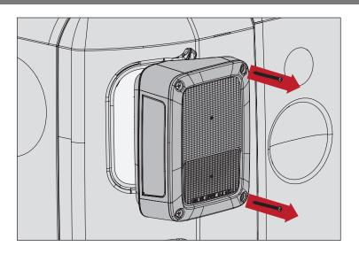
2. Disconnect taillight electrical socket. Push down on tab and pull connector apart.
