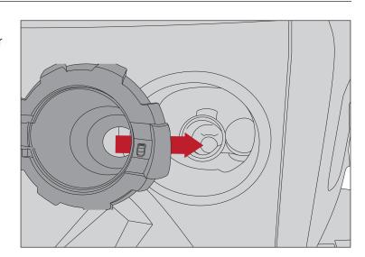
6. Reattach fuel door tether to Rugged Ridge Fuel Door filler housing.
