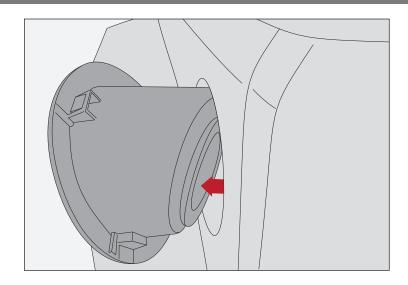
5. Align grommet on filler housing with fuel filler. Apply moderate pressure to front face of fuel door to engage.
