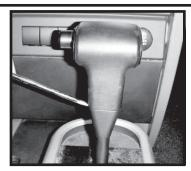
Step 2. Using a T15 torx bit remove the handle lock screw. Do not discard the screw it will be used to hold the new handle on. Once the screw has been removed slide the handle up and remove.
