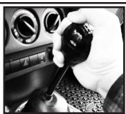
Step 2. Slide on your Rugged Ridge Manual Shifter and fasten it in using a 4mm hex key.
