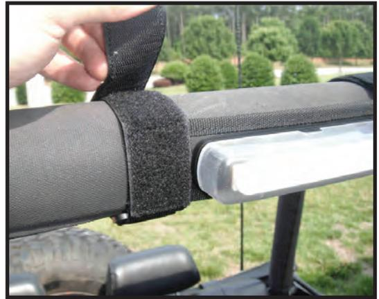
Step 2. Pull the slack out of the straps and wrap around to attach the strap.
