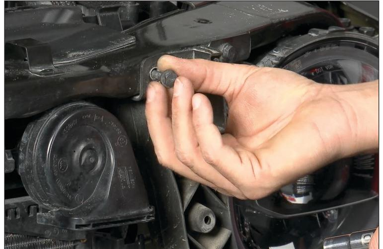
6. The new light bracket requires some pre installation of it's parts before attaching it to the Jeep. Take the Passenger side bracket and center bracket and loosely attach with provided hardware. The carriage bolt installs through the side bracket to the center bracket then a washer and serrated flange nut. There are two slotted locations on the side bracket to use for the selected lights you are using. Determine the correct location you desire and hand tighten the carriage bolt.
