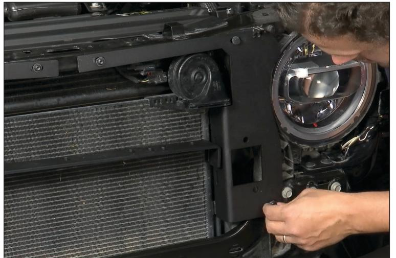
10. Install the carriage bolt on the Drivers side bracket through the center bracket, then washer and serrated flange nut. Adjust the center bracket the needed position, assure its level and fully tighten the bracket.
