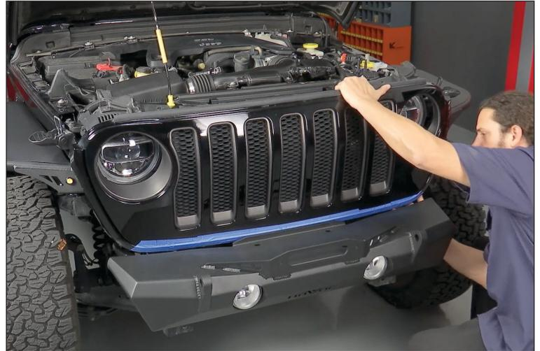
3. With grille removed notice the two support rods. Both these rods must be removed and can be disregarded. The rods are attached with a star torx screw. Keep these screws, they will be used to install the light mount.
