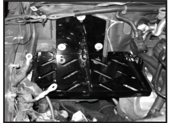
9. Install the front section of the factory battery box that was cut in step 6 using factory hardware. Then install the Fuse Box Bracket included with the Dual Battery Tray using the 3 Bolts and Flat Washers. The hinged factory fuse box bracket can then be installed on top of the Fuse Box Bracket included with the Dual Battery Tray. Reconnect all connectors to the fuse box and snap it back into position.
