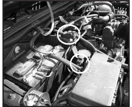
4. Remove the power steering reservoir bolt and move the reservoir to the side. Remove the reservoir mounting bracket and set aside.
