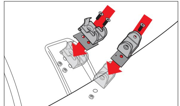
4. Re-attach the Aluminum Hood Catch assembly to the pivot base using the binding posts removed in Step 2.
