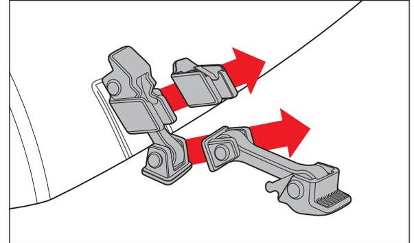
2. Remove the pivot base from the Aluminum Hood Catch assembly.
