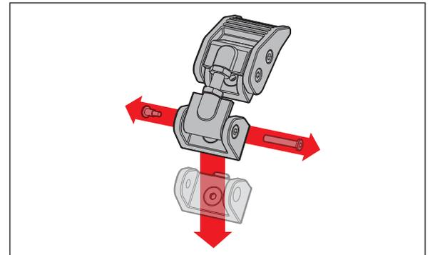
3. Fasten the catch to the hood. Fasten the pivot base to the fender.
