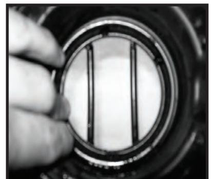
4. Reinstall fog lights and tighten all screws. It may be helpful to have someone hold the Euro Guards in place from the front of the bumper while the screws are tightened from the back.
