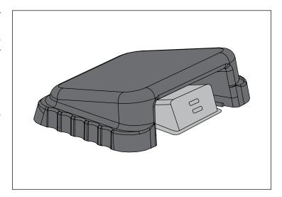
3. Remove stock bump stops from hood and clean area underneath. Install new Bump Stop, Base, and Gasket using supplied M8 hardware.
