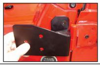
**Step 6.** Place the factory mirror onto the relocation bracket, taking care to align the mounting bolt holes. Using the included hardware, insert the bolts through the mirror and bracket mounting holes.
