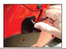
**Step 7.** Place one washer on each bolt, followed by one nut (included). Tighten the nuts snugly, taking care not to over tighten.
