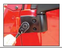
**Step 4.** Tighten both bolts snugly.
