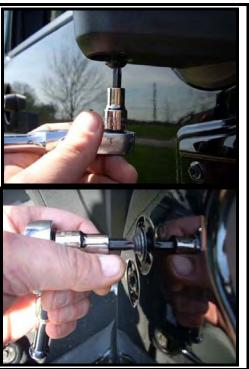
**Step 3:** Remove the front 2 torx head bolts from the windshield retainer bracket.
