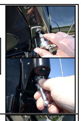
**Step 5:** Install the door filler plate, again working through the open window.
