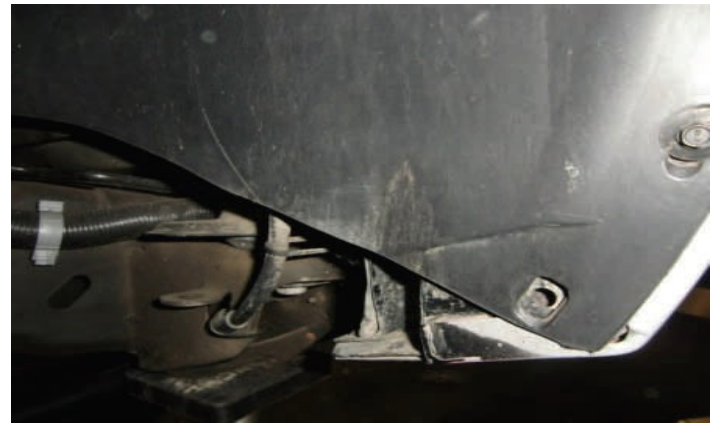
Slight/moderate trimming may be necessary for tire clearance
