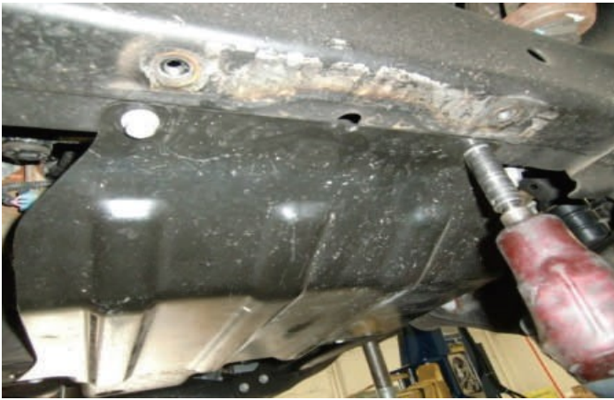
Reinstall front skid plate
