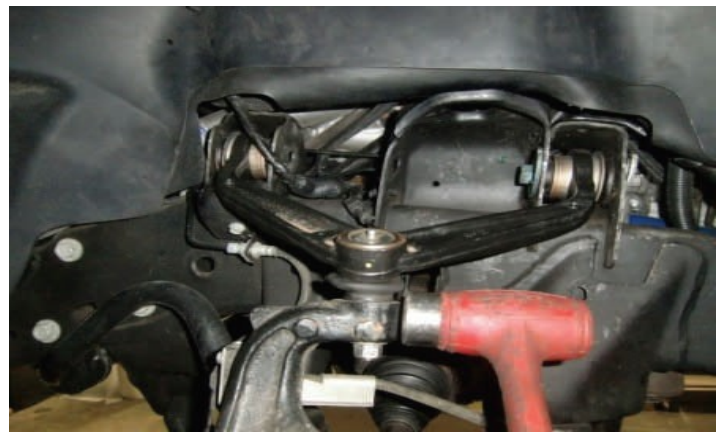
Strike spindle to disconnect ball joint from upper control arm
