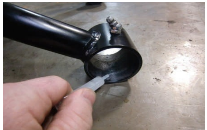
Install zerk fittings and apply grease to pivot tubes
