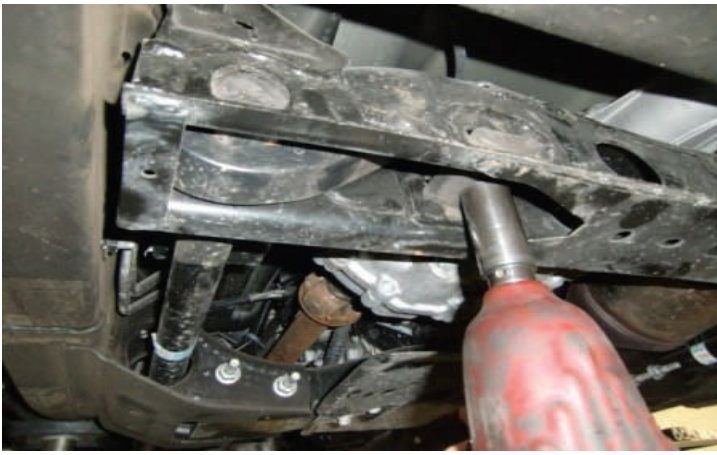
Remove torsion bar adjuster bolt. Set aside for later reuse.
