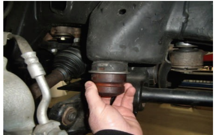
Remove factory lower control arm bump stops (4)
