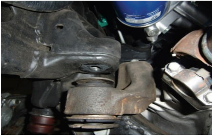
Support differential and remove (4) differential mounting bolts at frame. Lower the differential.
