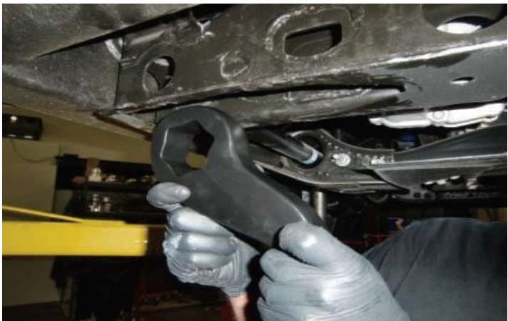
Install new torsion key and slide bar into position
