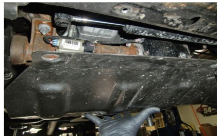
Remove skid plate bolts and skid plate
