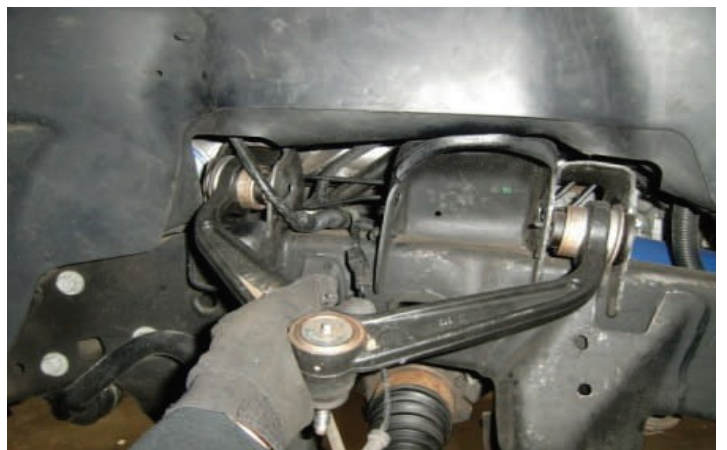
Remove upper control arm from frame pockets
