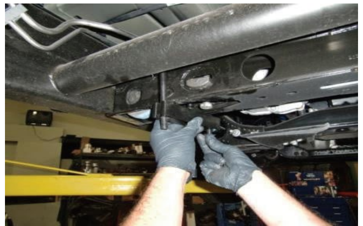
Position torsion bar unloading tool over cross member
