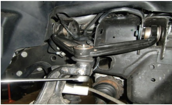
Loosen and remove upper ball joint nut.
