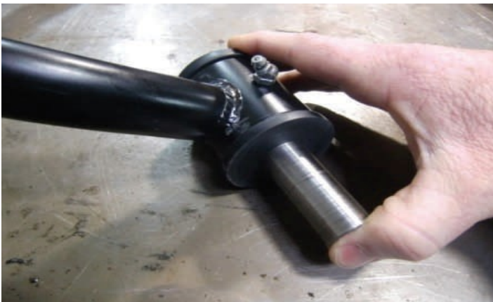
Assemble bushing halves and insert crush sleeves
