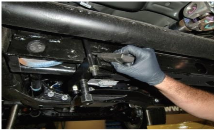
Adjust tool just enough to remove keeper block
