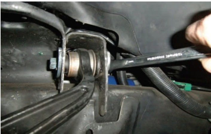
Loosen and remove pivot bolts and cams.
