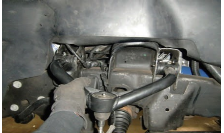
Install new upper control arm assembly with OE hardware
