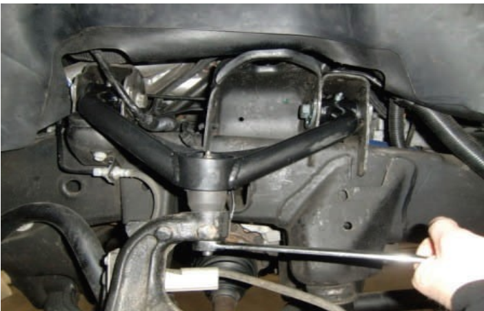
Connect upper ball joint to spindle
