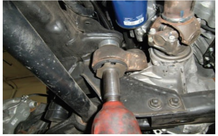
Install (4) differential drop spacers with new hardware
