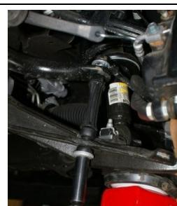
20. Re-attach the brake line bracket to the control arm and insert the wheel speed sensor cable into each of the factory harness clips. Repeat steps 3-20 on driver side. Make sure all hardware is tight and torqued to factory specs. Install the front wheels and torque the lugs to factory specs. Lower the vehicle and install the skid plate.
