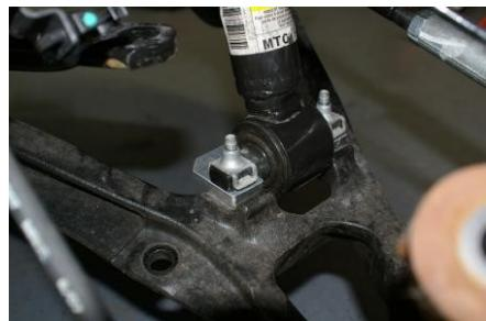
15. Position the strut and nut clips over the spacer and install the factory bolts to permanently secure the assembly.
