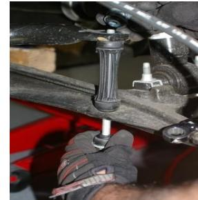
8 & 9. A 15mm socket is used to remove both lower strut mount bolts. Be sure to support the lower control arm before remove the bolts.
