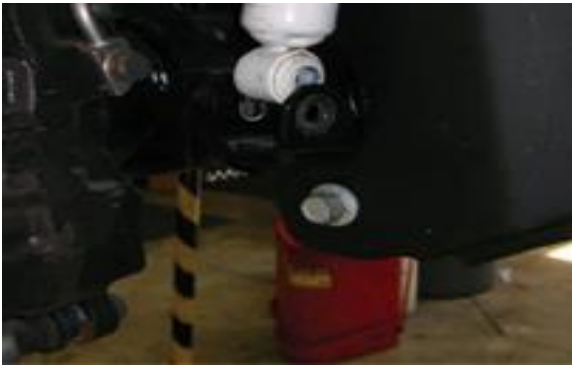
Disconnect dr./pass. front lower shock bolts
