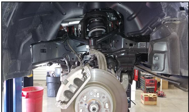
Install the upper control arms to the frame. Install the completed strut assembly to the frame using the provided hardware. Install the lower strut hardware.
