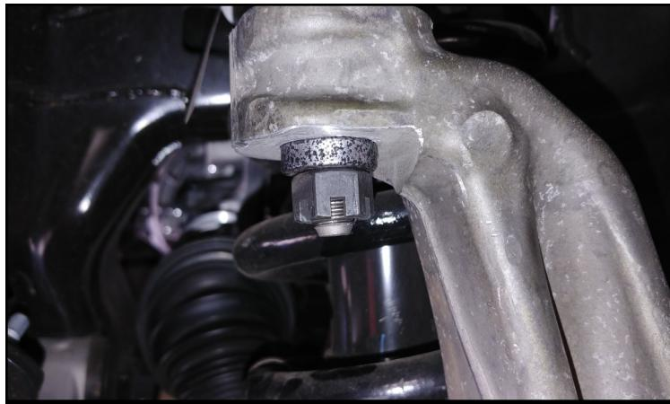
Install the upper ball joint to the knuckle using the supplied spacer and nut. Once tight, install the supplied cotter pin.
