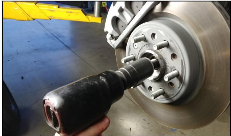
Remove the axle nut from the hub.
