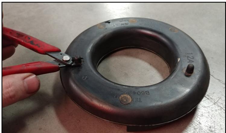
Cut off the nipples from the spring isolator.
