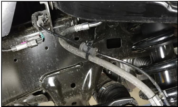
Install the brake line bracket onto the frame. Zip tie the ABS wire to the rubber brake line. Install the ABS wire into the clip on the rubber brake line. Reinstall the axle nut.
