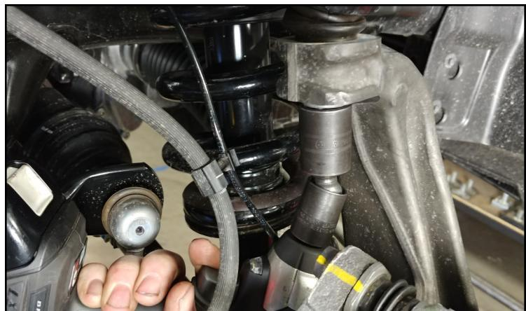
Remove the upper ball joint from the knuckle. Let knuckle hang out of the way. Do not stretch the ABS/brake lines.
