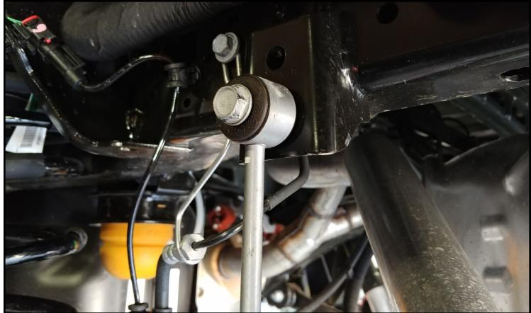
Remove the ABS wire and brake line from the frame. Remove any wire harness from the rear pumpkin to gain slack. Remove the sway bar end link from the frame.
