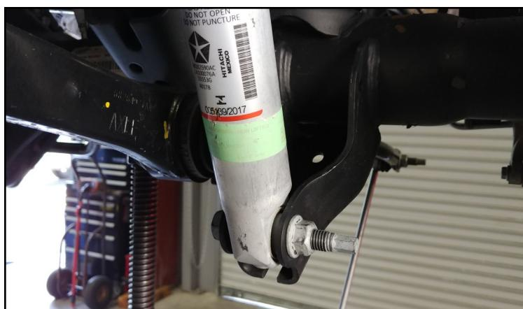
Loosen all control arms and track bar. Remove the lower shock hardware. Lower the axle down to remove the springs. Do not stretch the ABS, brake lines or any other harness.
