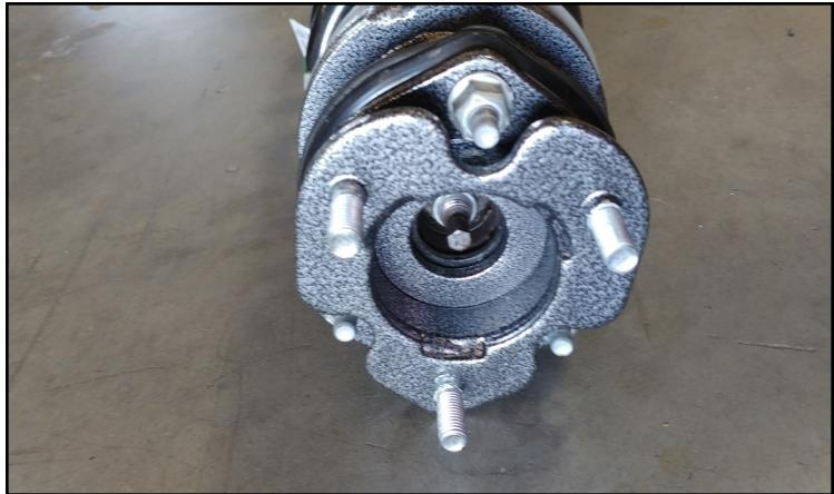
Install the strut extension to the strut using the factory nuts.
