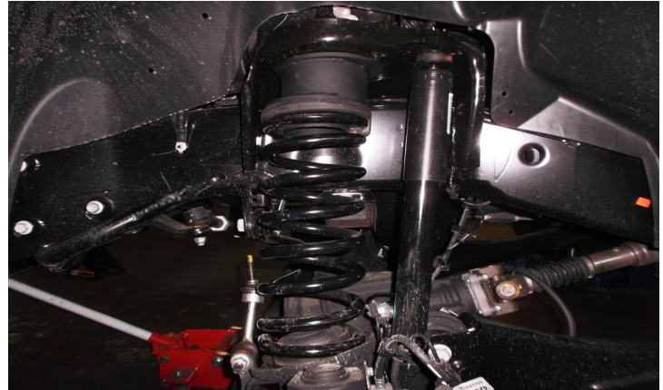
Raise the axle to weight the springs.
