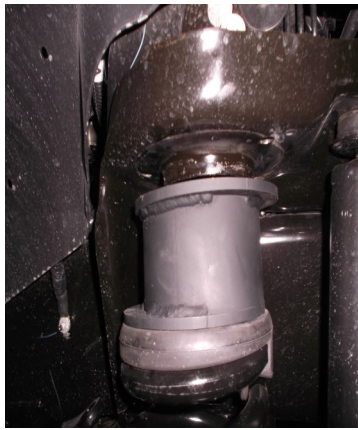
Install the assembly in to the vehicle. Note: Coil Spacer Should be orientated so the spring is offset to the front of the coil pocket and to the inside of the frame to correct "Spring Bowing"
