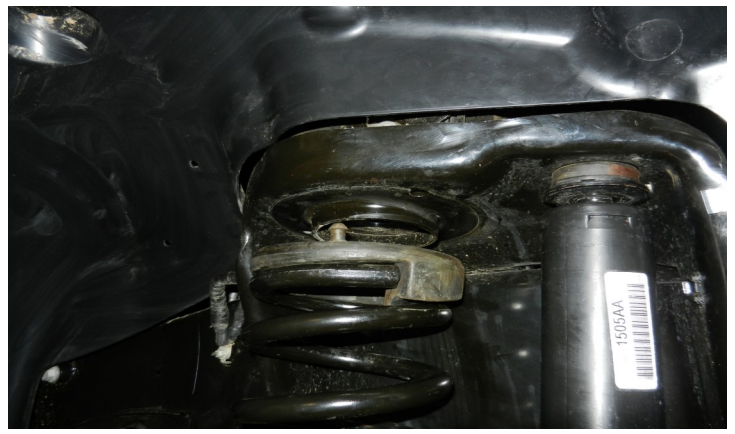
Lower the axle down to allow the front coil springs to be removed.
