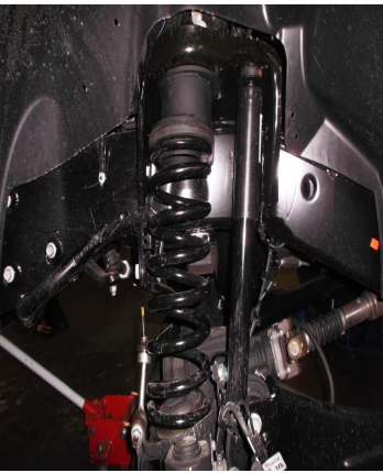
Install the assembly in to the vehicle. Note: Coil Spacer Should be orientated so the spring is offset to the front of the coil pocket and to the inside of the frame to correct "Spring Bowing"
