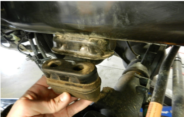
Remove the factory bump stops from the frame.
