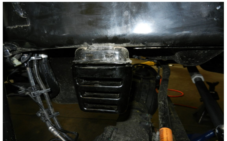
Install the 3" bump stops.
