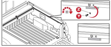
FOR 05-15 TACOMA INSTALL - Lower the tailgate and place the tailgate extrusion (R) assembly onto tailgate.
