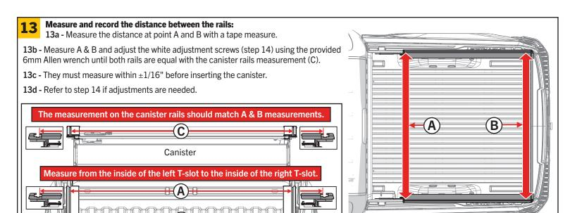
Adjust the distance between the rails: If A & B do not equal C in step 13, adjustments are needed using the following step. Remove the clamps and turn the white adjustment screws with the 6mm Allen wrench (J) to move the rails. One complete turn =1/16". Turn both screws. NOTE: When properly adjusted, replace the clamps as in steps 12. Make sure the clamps are tight.
