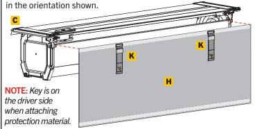
Canister preparation - attaching hook and loop to canister:
