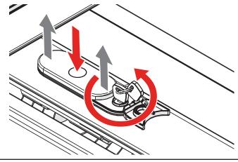
**CLOSING AND LOCKING THE COVER:** To latch your cover anywhere along the rail, push down firmly on the pop up latch. You can lock this location by opening the lock cover, inserting the key and turning it to lock the cover in place.
