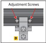
12b - The adjustable-back clamp is designed and tested for the extra loads for the retractable cover. The adjustable-back clamps must be positioned correctly under the truck bed rail to properly carry the extra loads.
