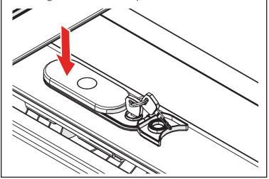
**LOCK COVER ADJUSTMENT:** A 3/32" Allen wrench can be used to adjust the pointed set-screw on the lock arm. Turn clockwise to increase latching pressure on the rail, or turn counter-clockwise if the lock is too hard to close. Use the same method on passenger side jam nut.
