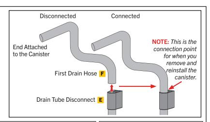
21b - Make sure the hoses and disconnect are running vertical, no kinks. Once you have the right length of both hoses and you find the right location that will be accessible under the canister, attach the drain tube disconnect to the truck using method A or B on driver and passenger sides. The drain tube disconnect allows you to remove the canister easily.
