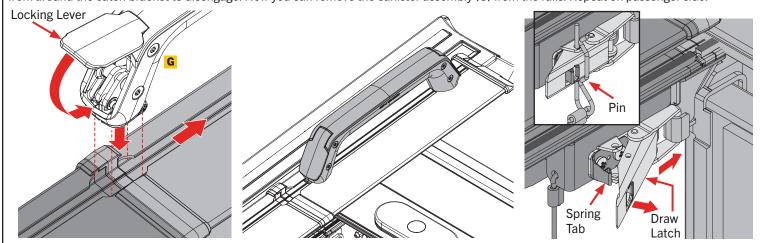
the cover is rolled up into the canister and the latch is closed. With two people using the lift handles (G), lift the canister assembly (C) out of the mounting bracket boot retainer feature first as shown below on both driver and passenger sides on to the bed of truck.
