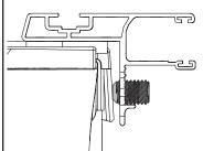
If the rails measured too close together, turn the screws counter clockwise.
