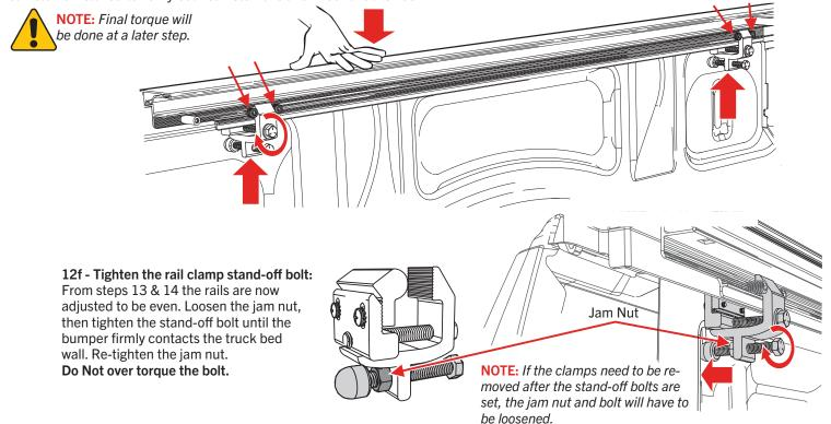
**NOTE:** Ensure the rails are parallel. If the rails are leaning down, have one person stand on the outside of the bed and slightly roll the rails upward while another person slowly snugs the clamps up. If the clamps are tightened too quickly or overtightened, it will cause the rails to lean down.
