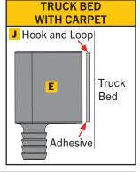
**20b** - Insert the loose end of the second drain hose into the hole of the truck bed floor before attaching the tube disconnect (E) to the truck to make sure you have enough hose length to allow the water to exit the bed (location varies per truck). Then see if the drain tube disconnect reaches to where you want to attach it. **NOTE:** You may need to cut the desired length of each drain hose to prevent kinks in the drain hoses.
