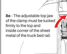
**8f** - If the jaw does not contact firmly into the corner of the bed flange, remove the clamp and loosen the screws to adjust the jaw.
