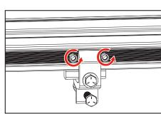
er, turn the screws counter clockwise. If the rails measured too far apart, turn the screws clockwise.
